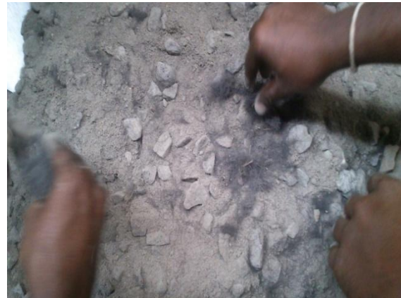
fig 2.1.5 - human hair used as a fibre
