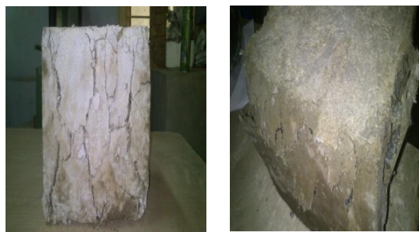
Fig 3.1.2 compression test specimens after test
